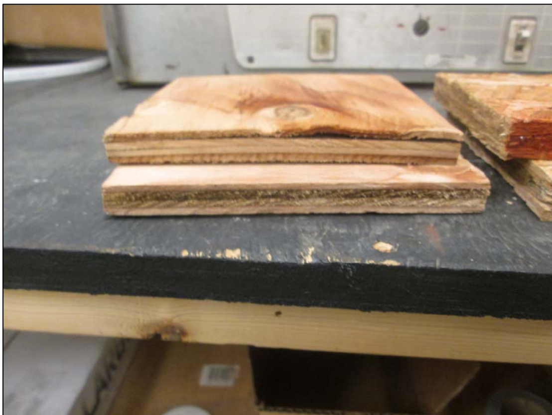
Photo 2. After 10 Cycles of Freeze-Thaw: Plywood
