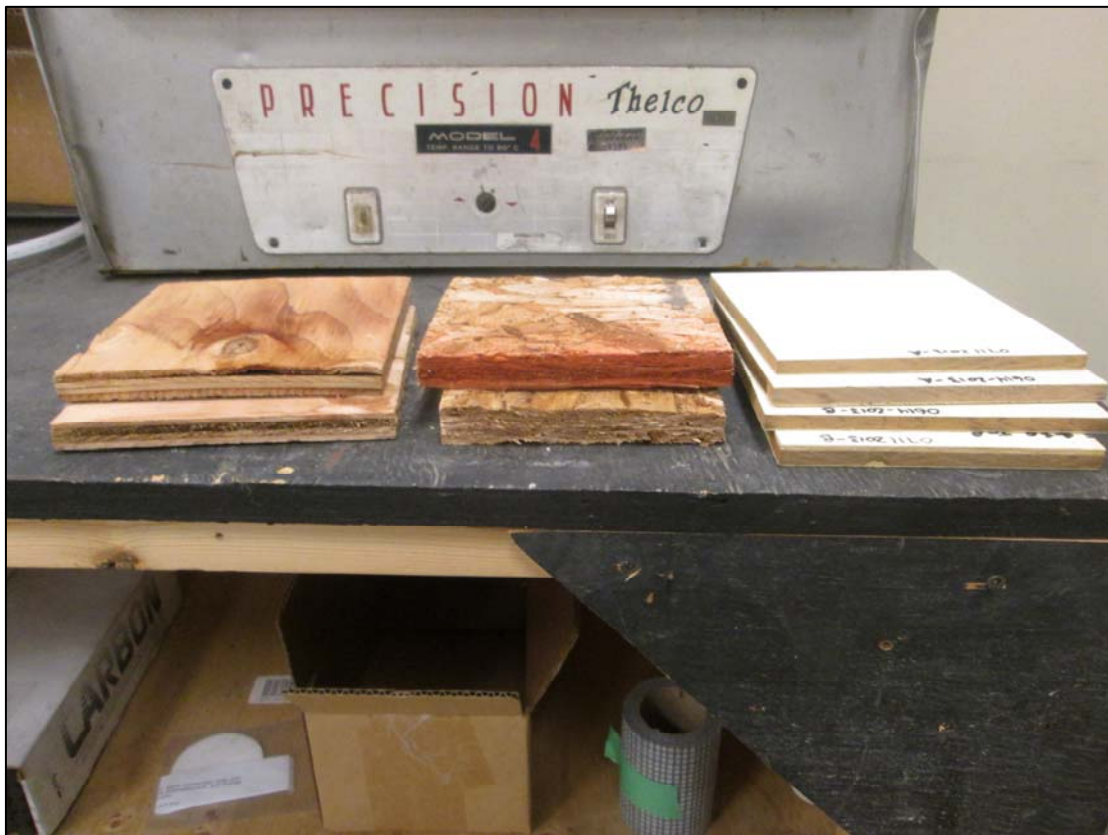
Photo 1. After 10 Cycles of Freeze-Thaw
