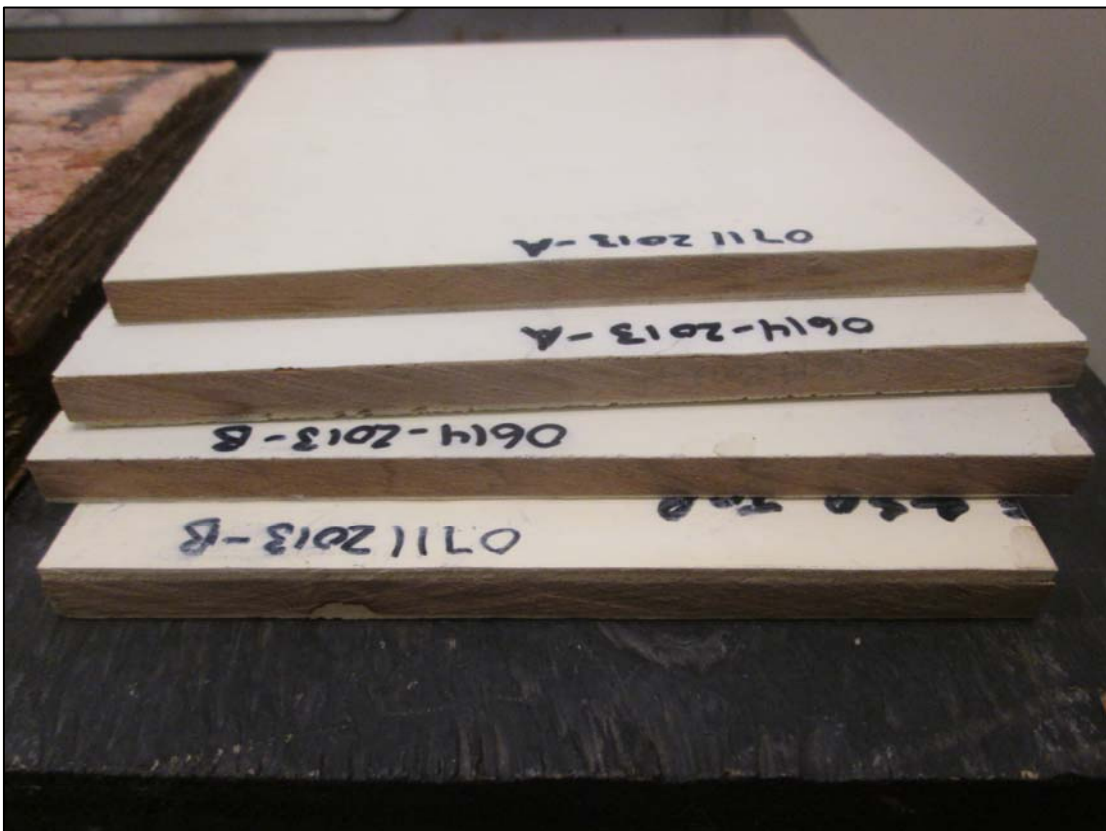
Photo 4. After 10 Cycles of Freeze-Thaw: Solid Wood Composite (SWC) Panels
