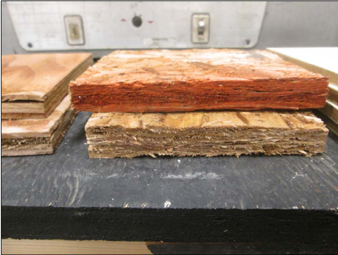
Photo 3. After 10 Cycles of Freeze-Thaw: OSB
